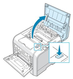
**5** Locate the jammed paper, and then carefully take it out of the printer.
